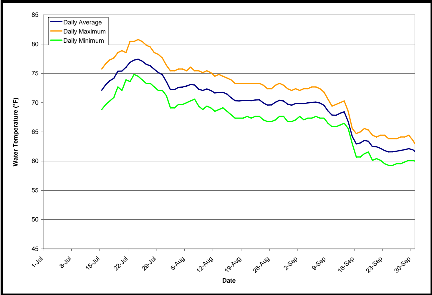
Figure 4. The daily average, maximum, and minimum water temperature recorded in the Rubicon River upstream of Ralston Afterbay (RR0.7) during July 1, 2006 through September 30, 2006.
