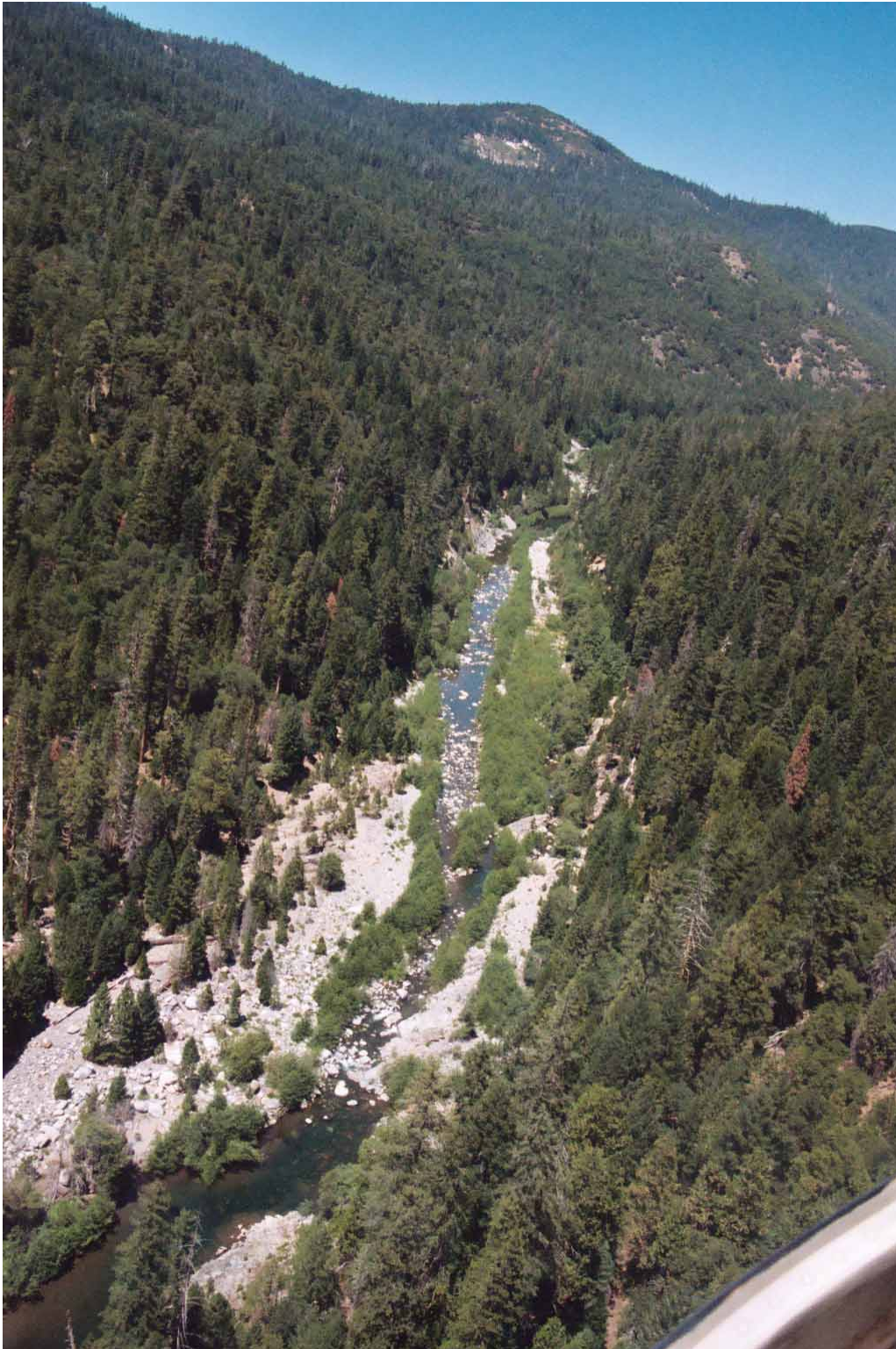
Photo F-7: Rubicon River (RM 26.0) Rosgen Level 1 B-channel type with a moderate entrenchment and width-depth ratio
